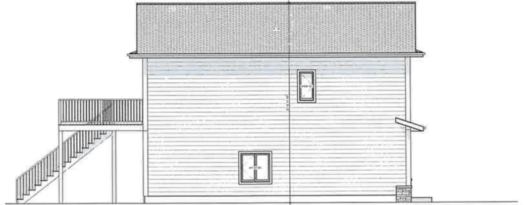
2 A3 LEFT ELEVATION SCALE = 3/16" = 1'-0"
